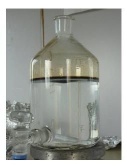
Figure 2: Preparation of an oil WAF
