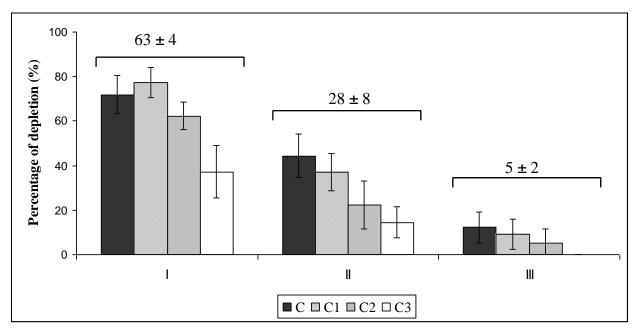
Figure 7. Degradation of chrysene (C) and some of its alkylated derivatives (C1, C2 and C3 refer to methyl-, dimethyl- and ethyl-, and trimethyl-, methyl-ethyl and propyl-chrysenes, respectively) in oil samples from Groups I, II and III. The number above the brackets represents the mean and standard deviation of percentage of degradation of total chrysenes (C + C1 + C2 + C3).
