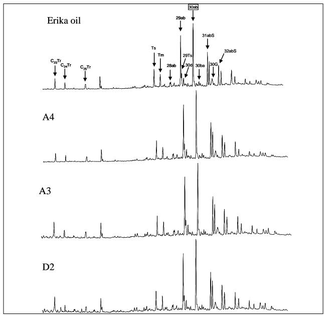
Figure 2. GC–MS chromatogram illustrating the preservation of biomarker terpanes (m/z 191) between the original Erika oil and samples (A4, A3 and D2) collected 10 years after the oil spill. (30ab was used as an internal standard).
