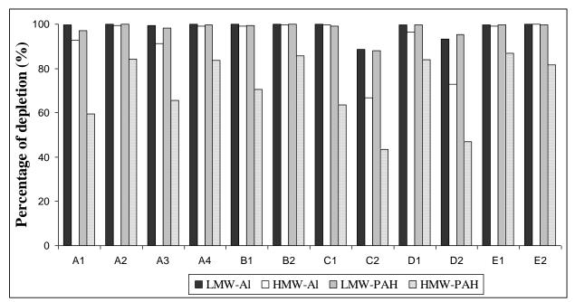
Figure 5. Degradation of low and high molecular weight *n*-alkanes (LMW-Al and HMW-Al) and low and high molecular weight PAHs (LMW-PAH and HMW-PAH) for samples of oil collected ten years after the Erika spill at different site locations (site A, B, C, D and E).
