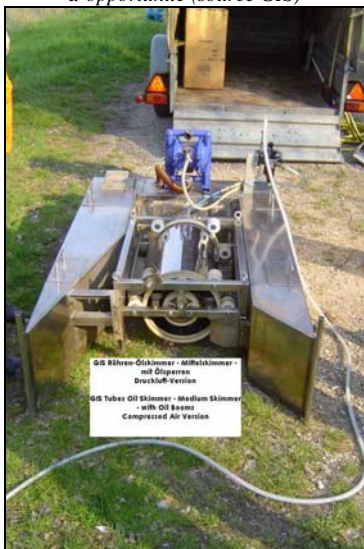
GIS Tubes Oil Skimmer (source GIS)
