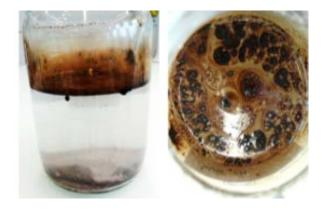
Sinking capacity: Marine water, simulated swell (200 RPM), 2h
